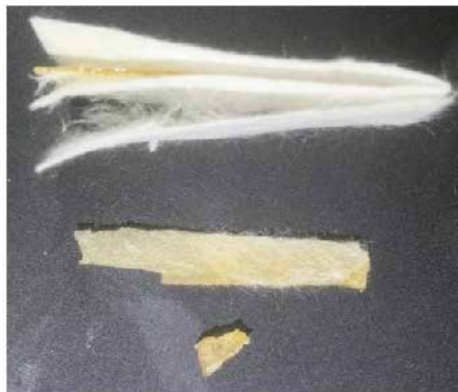
Figure 7: The unknown polymer in filter membrane. The membrane fibers were removed with a file to analyze the unknown polymer in the DSC.
