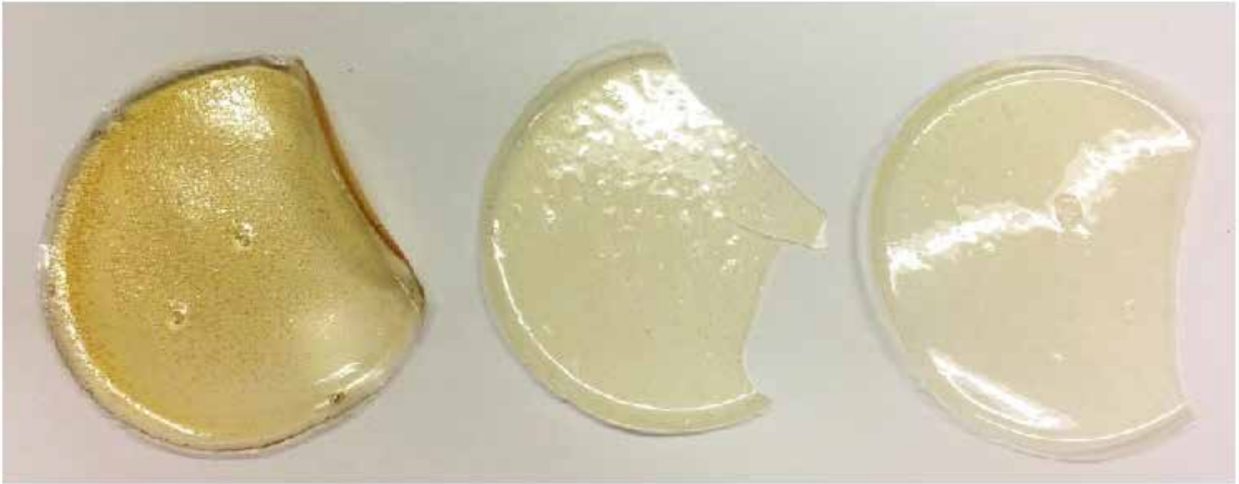
Figure 8: Oven Cured 7g Samples. Samples 1-3 are laid out from left to right. Sample 1 was bent over to show ease of deformation. Samples 2 and 3 show cracking and were brittle.
