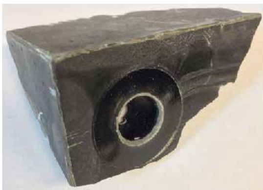
Figure 6: A sample of the polyurethane molded cover used in electrical transformer housings.
