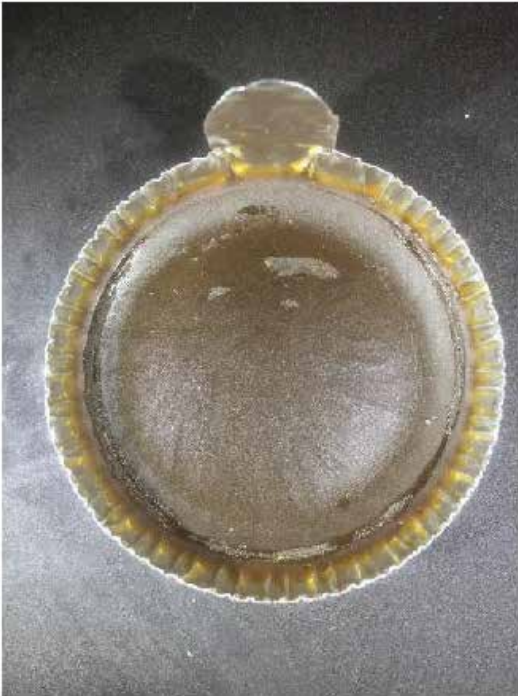
Figure 4: An example of hydrocarbon-based binder used in equine sport track surfaces produced from Soxhlet extraction.
