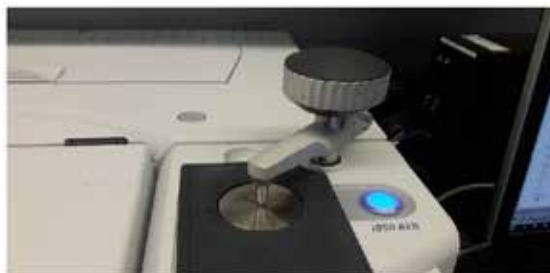
Figure 4: Diamond crystal for the Thermo – Nicolet iS50 FTIR – ATR.
