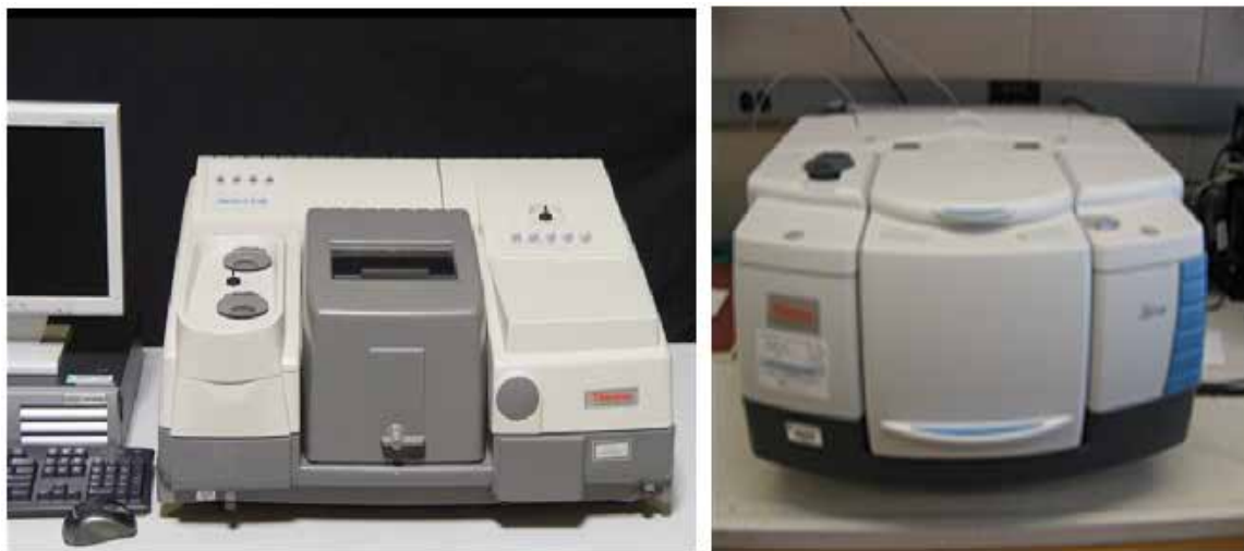
Figure 3: Thermo Scientific Nicolet 380 (Left) & Nicolet iS50 (Right) FTIR Spectrometers used at UW Bothell.
