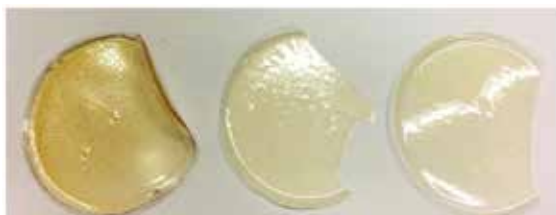
Figure 7: Oven Cured 7g Samples. Samples 1-3 are laid out from left to right. Sample 1 has been bent over to show ease of deformation. Samples 2 and 3 show cracking.
