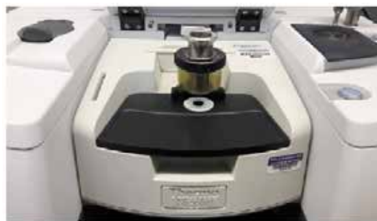
Figure 5: Germanium crystal for the Thermo- Nicolet iS50 FTIR – ATR
